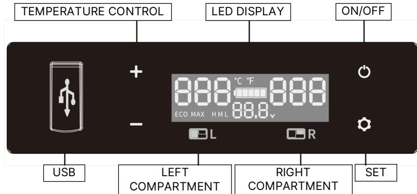
\* Note: The right compartment is on the side where the compressor is.
