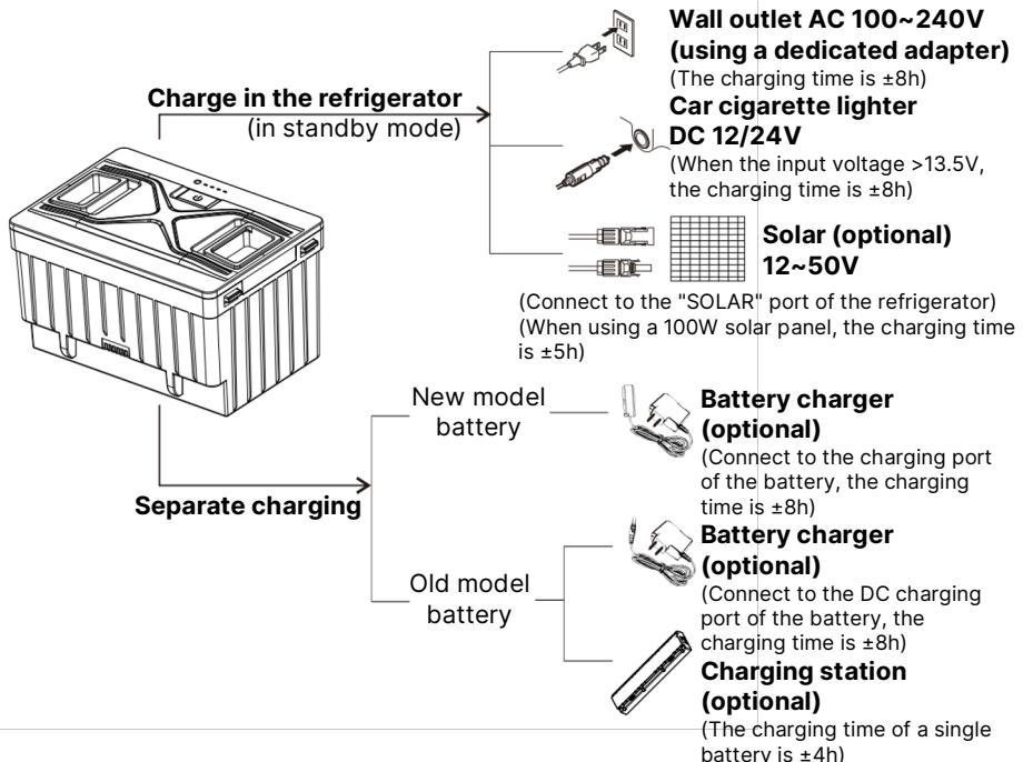
**Note:** It is suggested to switch off the refrigerator when charging the battery (the power supply may mainly power the compressor when the refrigerator is running). When connected to a solar panel, please place the refrigerator in a cool place to dissipate heat.
